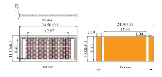
**Note:** Soldering procedure: The base plate is at right angles, and there is no bevel or chamfer. The copper clad and the substrate copper cannot be layered for 30 minutes at 300 degrees
