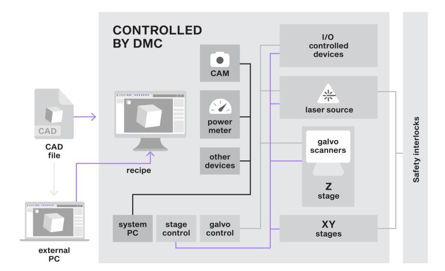
DMC software controls complete laser machine, including:
