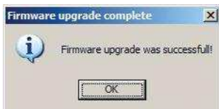
Figure 17. Normal firmware update process finish is indicated by “Firmware upgrade complete” message.
