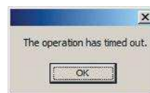
Figure 20. Error, thrown if device firmware becomes corrupted.
