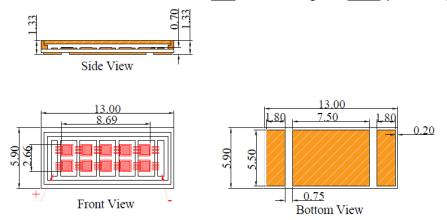
VD-0808I-50W-6K-3A0 with Substrate 6=Cu and Package K=T-mount (unit: mm)
