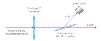
**Figure 1.** PowerXP operation principle. The intensity of the incident beam is varied by means of a  $\lambda/2$  phase waveplate and a polarizer.
