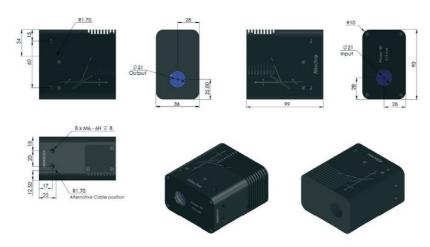
Figure 13. Main dimensions and mounting options of PowerXP.
