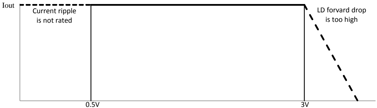
Fig. 1 - output characteristics of laser diode driver
