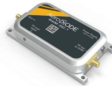
RF Driver - std version (TTL or analog).
