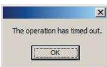
Figure 38. Error, thrown if device firmware becomes corrupted.
