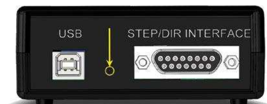
Figure 37. “Firmware upgrade” button location inside Watt Pilot controller.
