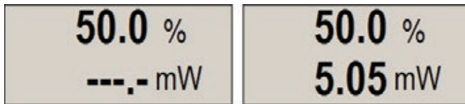
Figure 6. Power meter panel: right - “Use absolute power measurement units” checkbox is set in “Options → Preferences”, left - checkbox is unset.
