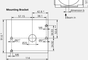
Standard mounting bracket (10 mm aperture): rectangular, without cut-out
