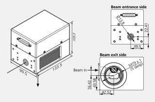
The housings of the SCANcube  $^{@}$  III series are identical with those of the SCANcube  $^{@}$  scan heads.
